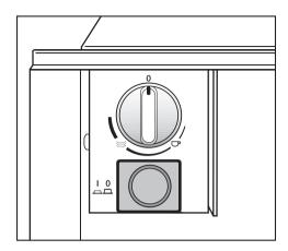
The controls consist of the temperature selector and the On/Off button. They are only visible when the drawer is open.
